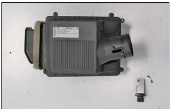
15. Remove the mass air sensor from the factory air box.
