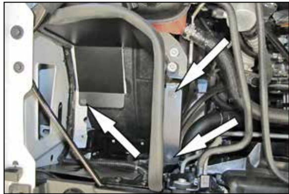
9. Install the heat shield assembly and secure to the air box mounting plate location using the three factory bolts from step #7.
