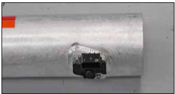
16. Install the mass air sensor into the K&N intake tube and secure with the provided hardware.
