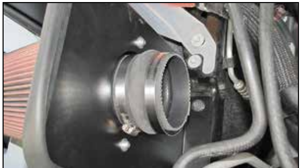
14. Install the coupling hose (08699) to the filter adapter and secure with the provided hose clamp.
