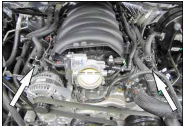
12. Remove the two factory crank case vent tubes from the vehicle.
