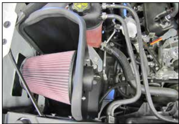
11. Install the filter assembly into the heat shield filter top first, then rotate the filter and pass the adapter through the hole in the heat shield. Secure the filter adapter to the heat shield using the provided hardware.
