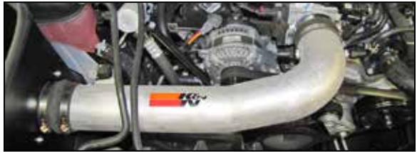
18. Install the K&N intake tube into the hose at the filter adapter and then into the hose at the throttle body, adjust the tube for best fit and then secure with the provided hose clamps.
