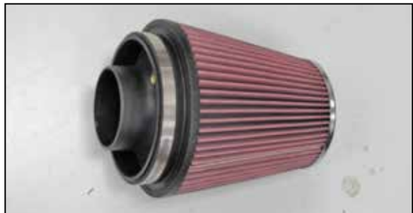
10. Install the filter adapter into the K&N air filter and secure with the provided hose clamp.
