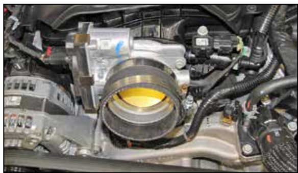
13. Install the coupling hose (08698 for 5.3L, 08497 for 6.2L) onto the throttle body and secure with the provided hose clamp.
