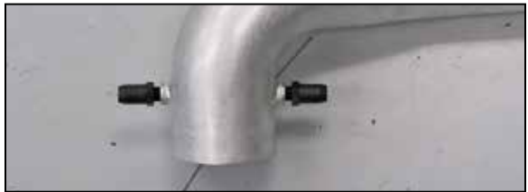
17. Install the two provided crank case vent fittings into the K&N intake tube as shown. NOTE: NPT fitting has tapered threads and only designed to be installed until hand tight, then tighten one rotation or when the fitting becomes difficult to return.
