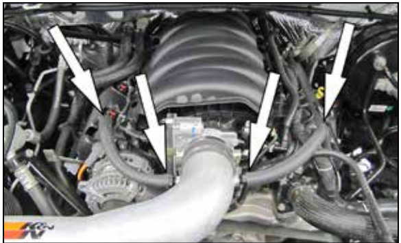
19. Connect the provided crank case vent hoses to the ports on the valve covers and then connect the open ends to the fittings installed into the K&N intake tube and secure with the provided hose clamps.
