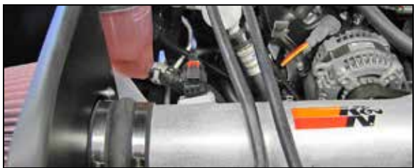
20. Reconnect the mass air sensor electrical connection.
